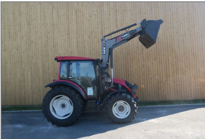
MX equipment : U306 on A94
