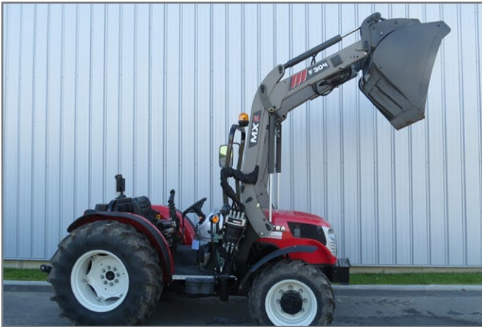
MX equipment : F304 on A73F
