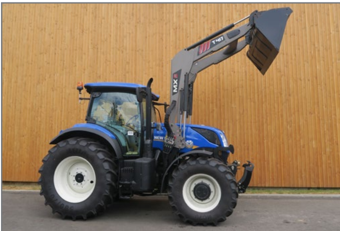
MX equipment : T417 on T7.165S
