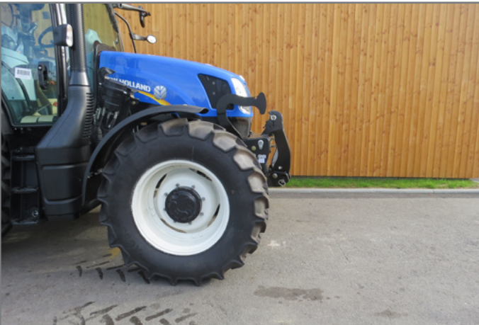
MX equipment : R28 on T6.150
