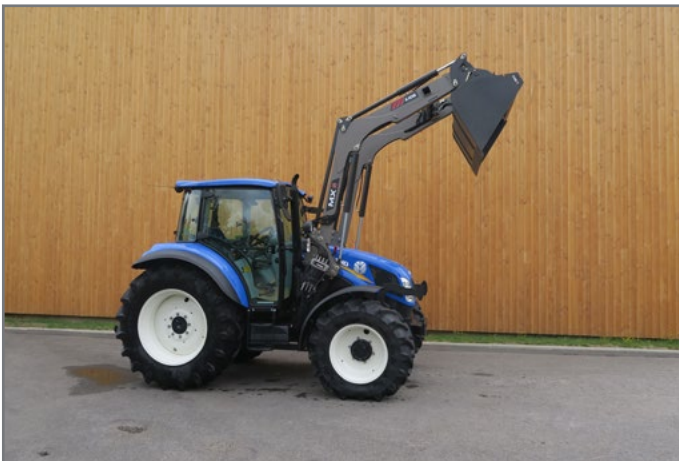
MX equipment : A106 on T5.95
