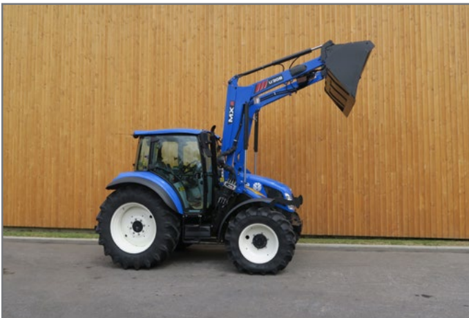
MX equipment : U308 on T5.95
