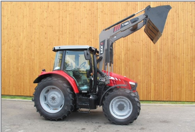
MX equipment : T410 on 5712 SL
