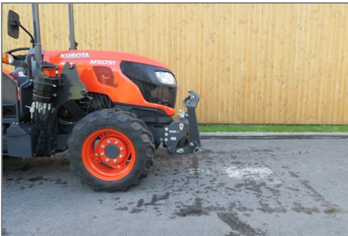
MX equipment : R16 on M5091N
