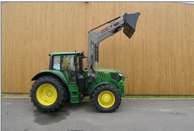
MX equipment : U414 on 6135M
