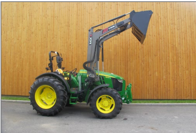
MX equipment : U308 on 5115M
