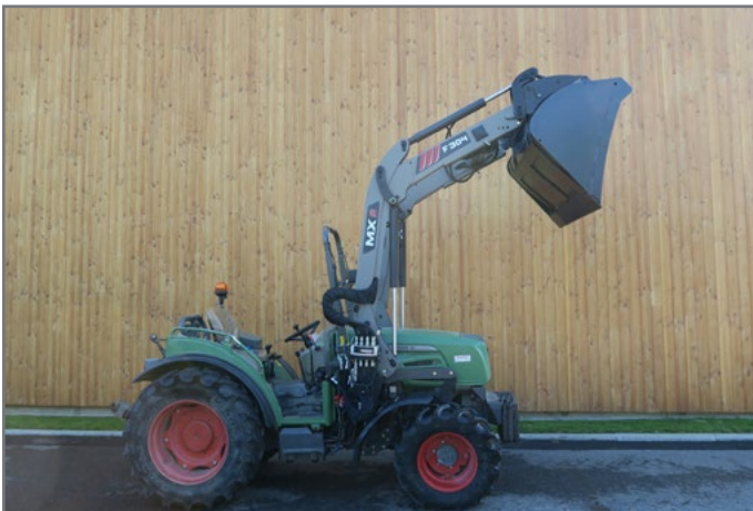
MX equipment : F304 on 206
