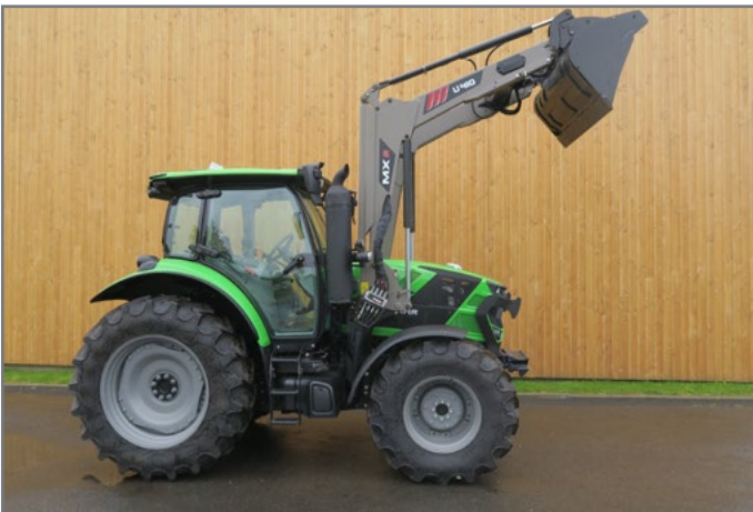
MX equipment : U410 on 6120
