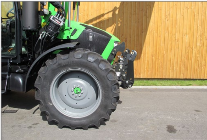
MX equipment : R28 on 5115
