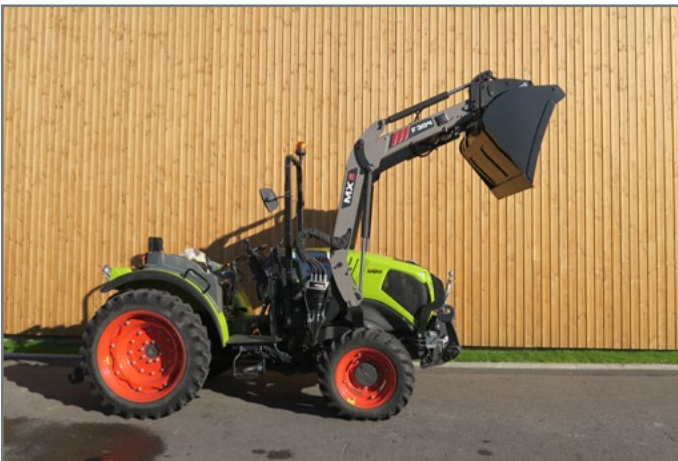
MX equipment : F304 on 210
